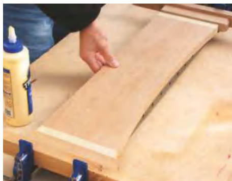
STEP 11. Cramp end pieces to the panel using PVA glue. I find masking tape makes cleaning up that much easier
